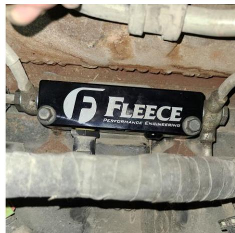
**STEP 12:** Re-install the two bolts securing the transmission isolators that were removed in STEP 6. Plug in the water in fuel sensor connector and reinstall the intake horn.
